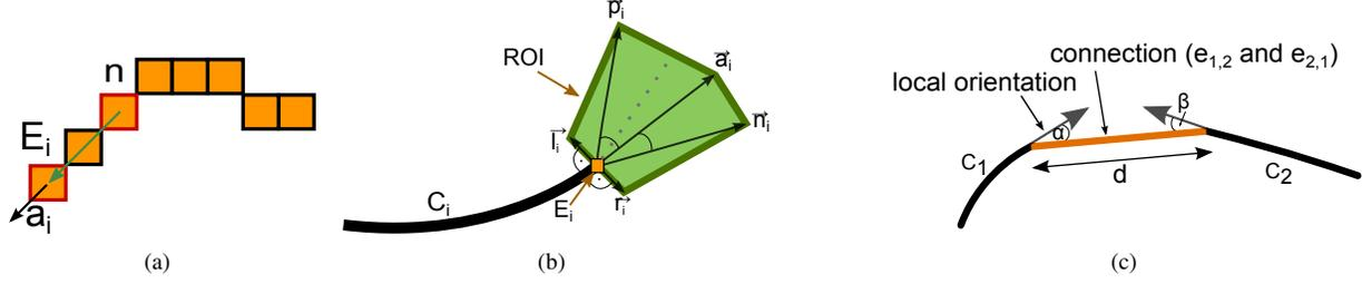
**Figure 2.** 2(a) illustrates the calculation of the local orientation vector. 2(b) and 2(c) show the definition of the search space used when searching for components to connect with, and an example of a connection between two components with distance  $d$  and the two angles  $\alpha$  and  $\beta$ , respectively.
