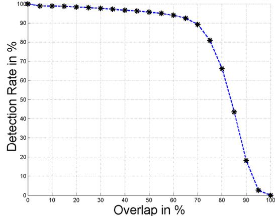
**Figure 6. Detection rates for different grades of overlap between ground truth and detected region**
