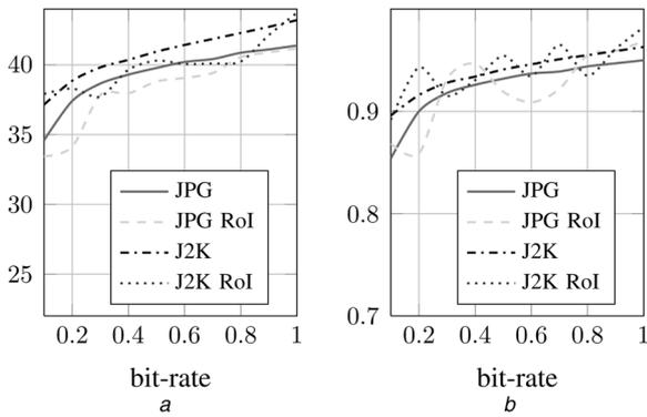
**Fig. 3** Quality estimation in terms of average PSNR and SSIM for original compressed images and according RoIs
