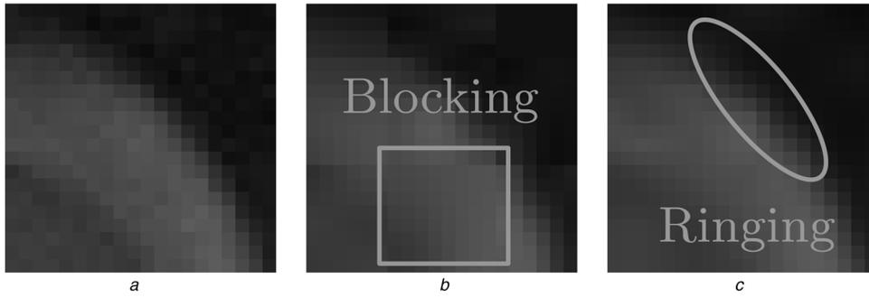
**Fig. 2** Comparison of artefacts:  $20 \times 20$  pixel patches at the helix of the ear of image ID 02463d002 at a compression rate of 0.2 bpp
