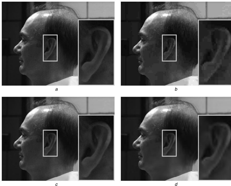
**Fig. 1** Sample compressions of image ID 02463d002 of the UND-J2 ear database [47] and close-ups of RoIs (at the right-hand side bottom of each subfigure) at compression rates of 1 and 0.1 bpp. Homogeneous regions within the original image (e.g. at the right-hand side top) allow for a more efficient image compression
